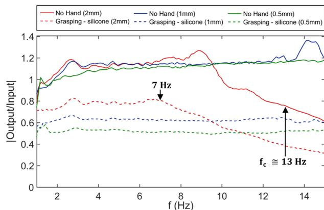
Fig. 5. Bandwidth results obtained through empirical transfer function estimate (ETFE). The corner frequency is at least 13 Hz in all displacement cases without grasping. With grasping, the bandwidth is clearly diminished, with the maximum displacement case worsening after 7 Hz.
