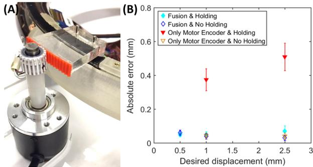
Fig. 4. (A) Set-up for position error test and bandwidth test. An external encoder was attached to the bearing to measure its absolute position. (B) Position control accuracy (average of absolute error and 95% interval)
