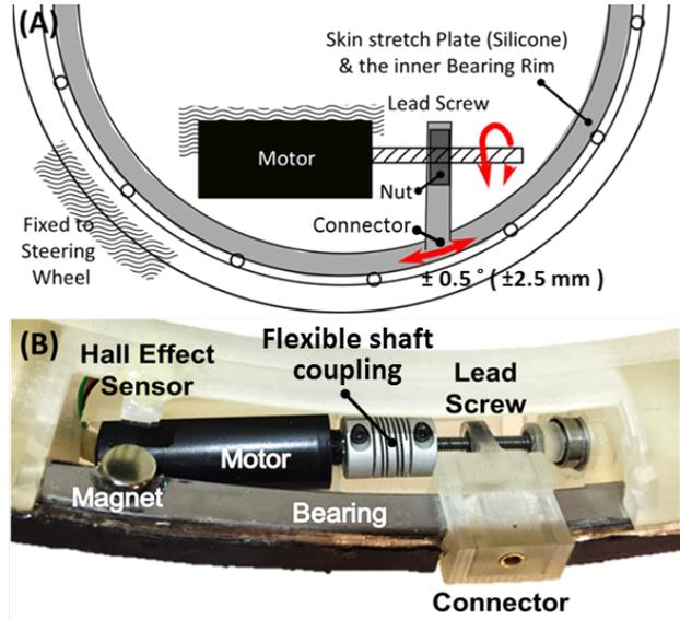
Fig. 3. (A) A screw and nut are mounted to a 3D-printed connector which is attached to the inner ring of the bearing to rotate it  $\pm 0.5$  degrees. (B) Close up view of the actuation and sensing elements, including a motor and flexible shaft coupling.
