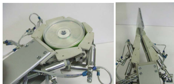
Fig. 10: The TWIX hand performing an enveloping grasp on the left and a fine pinch grasp on the right.
