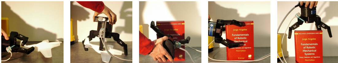
c) (from left to right) Two grasps of airplane model fuselage and three grasps of a book, each one obtained from a different approach direction.
