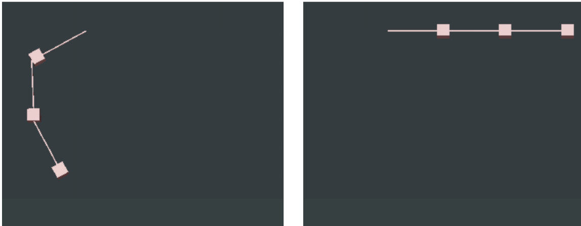
Figure 7-31: An example used to demonstrate springs and dampers. The sub-figure on the left shows the initial condition of the pendulum and the one on the right shows the resting configuration. This simulation is contained in the file “springPendulum.xml” in the examples directory.
