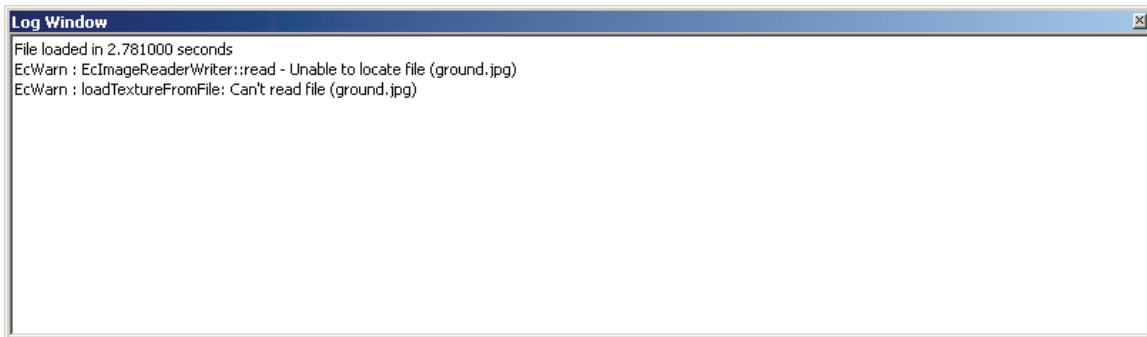
Figure 18-4: Floating EcLogPlugin window. It is useful to use this Plugin to determine if there are any problems with simulation files. Here a file gets loaded, but a reference to an image file cannot be found.
