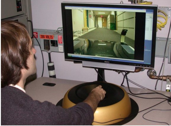
Fig. 7. Controlling RHex through the visio/haptic interface, showing a typical run through a hallway.
