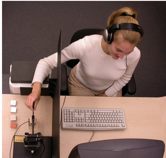
Figure 4.16: Setup for blind tapping on real and virtual wood.
