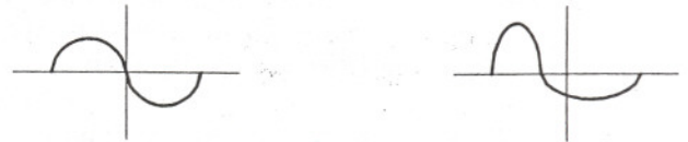
Fig. 17. Two functions that integrate to zero. One is symmetric and one is not. Symmetry provides a sufficient condition but not a necessary condition for zero net forward acceleration.
