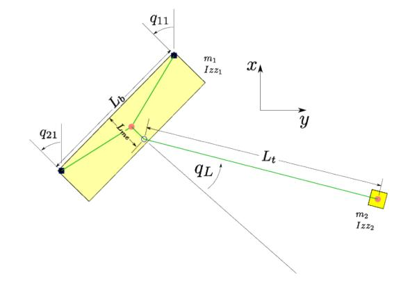
$\begin{array}{ll} m_1 & 0.335 \ kg \\ Izz_1 & 0.0032 \ kg \text{-}m^2 \\ m_2 & 0.3 \ kg \\ Izz_2 & 0.0 \ kg \text{-}m^2 \\ L_b & 0.305 \ m \\ L_{me} & 0.07 \ m \\ L_t & 0.457 \ m \end{array}$
