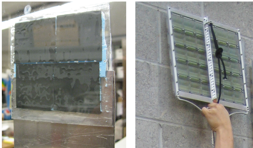
Figure 5.2: Left, example of a patch of dry adhesive supported by a hierarchy. The patch is viewed through the glass surface it is attached to, with gray areas attached and black areas not attached. Even with the hierarchy, the patch is only partially in contact with the surface. Right, a large patch with multiple rows of spines.
