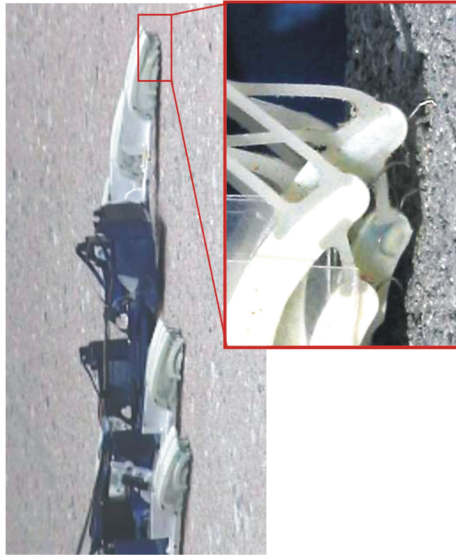
Figure 2.7: Picture of upper section of SpinybotII on concrete wall and detailed view of several spines independently engaging asperities on the concrete surface.
