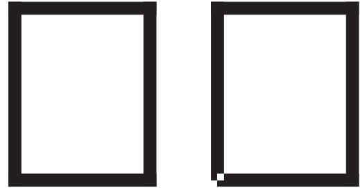
Figure A-7. Left = Closed polyline with width drawn in AutoCAD. Right = Mask data with notch due to self intersection.
