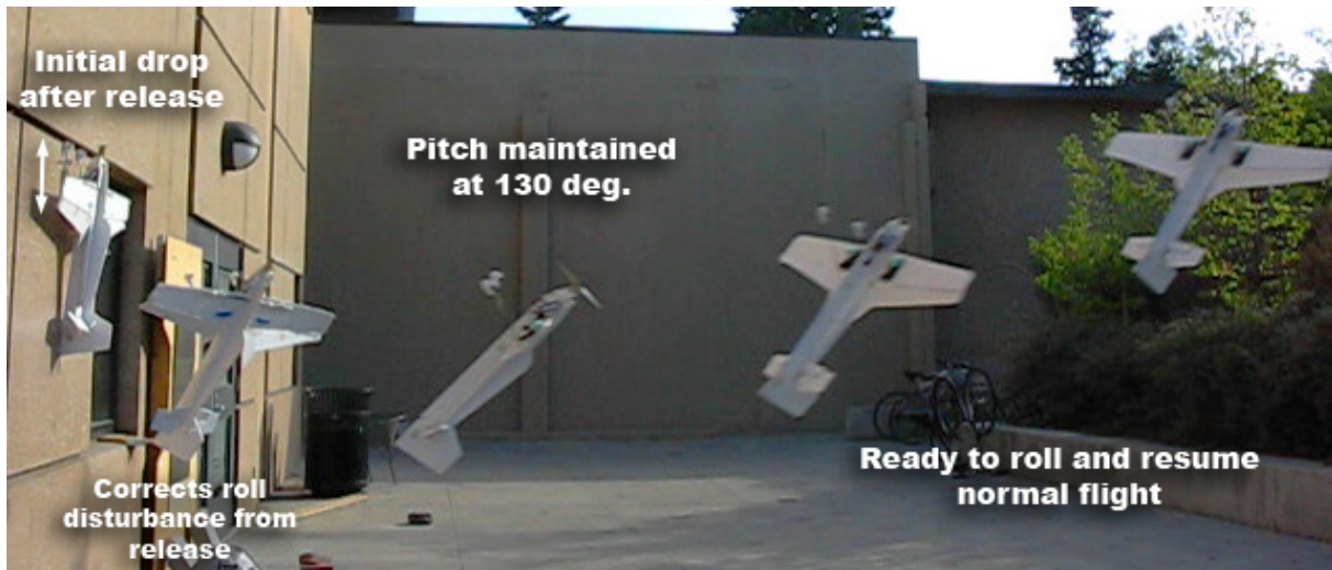
Fig. 4. Multiple exposure photography of the takeoff sequence. The airplane is originally at rest on the wall with ailerons and elevator ready for takeoff. The propeller is then commanded to a T/W ratio slightly less than 1.0; spines are released and the T/W ratio is increased to about 1.08 as the pitch angle is controlled to approximately 120 degrees from horizontal. Note that the spines have been intentionally released early in this example to clearly illustrate this step, but with ideal timing no vertical drop is observed.
