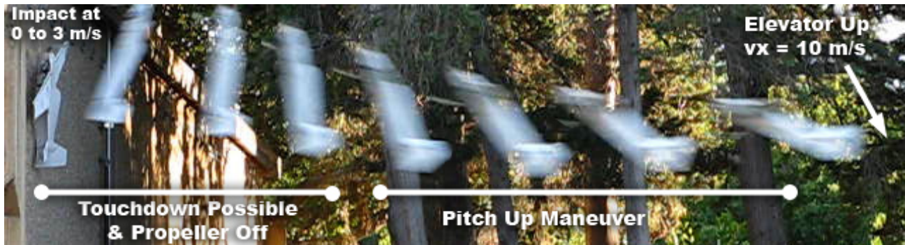
Fig. 1. Sequence of the plane performing a powered perching maneuver on a concrete wall. The plane is initially flying around 10 m/s, detects the wall at 6m and initiates a pitch up. The motor is turned off as soon as touchdown is possible, and the plane generally contacts the wall while moving at 0-3m/s in the horizontal direction. The landing gear finally absorbs the impact and engages the spines. The entire process takes < 1 sec.
