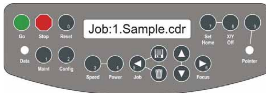
Control Panel – Key with numbers will be used to set the Ethernet IP Address.
