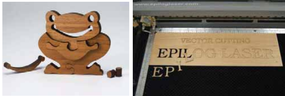
The two samples above show the results of Vector Cutting in wood.
