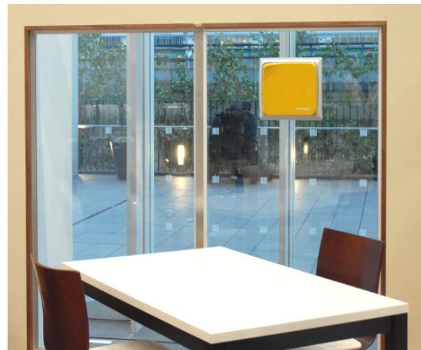
(a) A scene of WallWalker working on the window in the living room
