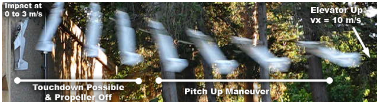
Fig. 1. Sequence of the plane performing a powered perching maneuver on a concrete wall. The plane is initially flying around 10 m/s, detects the wall at 6m and initiates a pitch up. The motor is turned off as soon as touchdown is possible, and the plane generally contacts the wall while moving at 0-2.7m/s in the horizontal direction. The landing gear finally absorbs the impact and engages the spines. The entire process takes < 1 sec.
