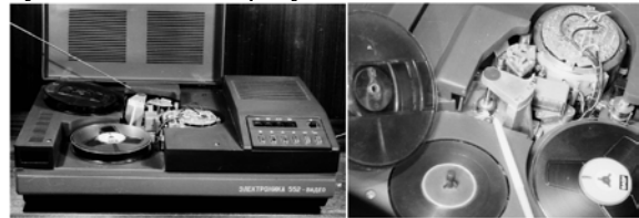
Fig. 12 Example of the "Elektronika 552-Video" a factory-built video recorder with an ultrasonic motor to power the drive axis, 1982
