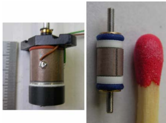
1994...2000 Fig. 28 Prototypes of miniature traveling wave motors from Physik Instrumente (PI)
