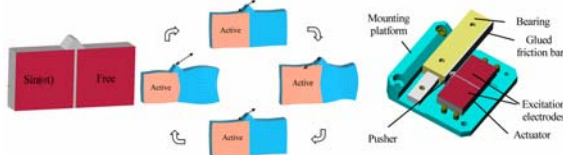
Fig. 20 Single-phase motor from Physik Instrumente (PI) with an asymmetric standing wave in the actuator plate, 2004
