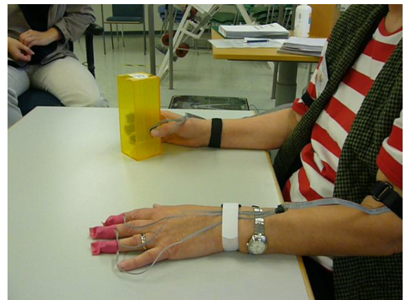
Figure 4. Experiment setup: force sensors are attached on fingertips of subject's right hand. Vibrotactile factors are attached on the fingernails of subject's left hand.
