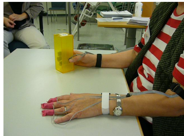
Figure 4. Experiment setup: force sensors are attached on fingertips of subject's right hand. Vibrotactile tactors are attached on the fingernails of subject's left hand.
