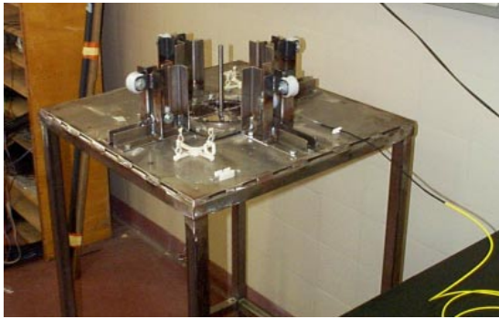
Figure 3. The calibration table allowing forces and torques to be applied. On the right, we see the single fibre connecting the sensor with its instrumentation.
