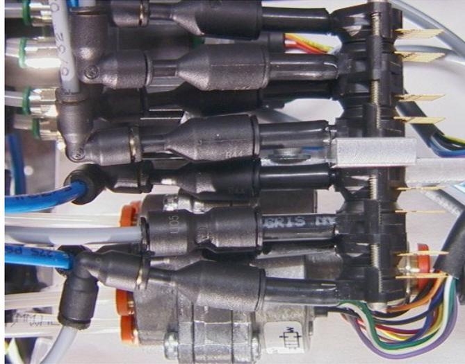
Figure 8.9: A pressure sensor array.
