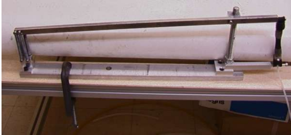
Figure 1: Actuator fatigue testing rig
