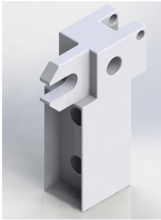
A second iteration of the brake finger design. The problem of low coefficient of friction was solved by designing a mold into the part and casting urethane into the portion of the finger that comes in contact with the acetyl and acrylic manipulator.
