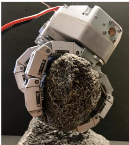
Fig. 1: SpinyHand grasping a pumice rock. The contact areas are covered in microspines to support large tangential forces.
