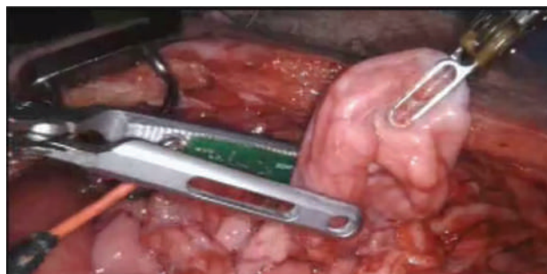
Fig. 4 In vivo porcine testing via laparotomy and da Vinci Xi Surgical System with prototype grasper (left hand) and Fenestrated Bipolar Forceps (right hand)
