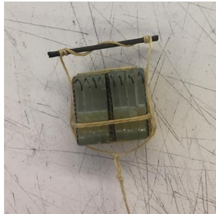
Figure 8. Third iteration of Super SCAMP Microspine design.
