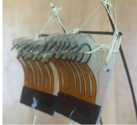
Figure 9. Final iteration of Super SCAMP Microspine design
