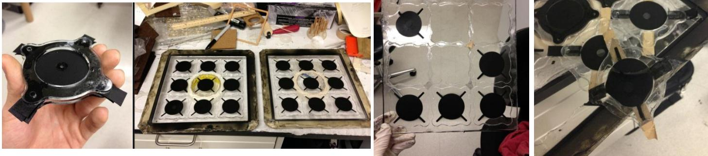
First method: using transferring frame to separate the acrylic film into independent areas for ceasing the tearing propagation ([Attach:Photo\\_transferring frame.png](#)).
