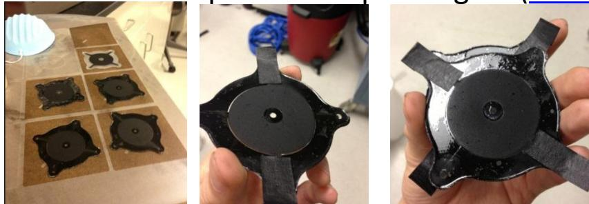
A supporting frame with flexibility (0.01" fiberglass currently, could be even thinner) can be much better and more easily glue on the acrylic film than rigid acrylic plate.
