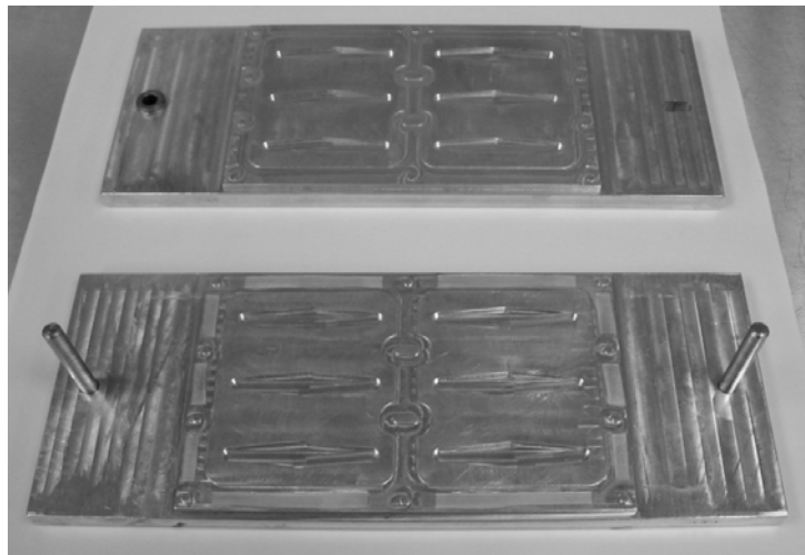
Figure 94: Interstitial frames assembly jig.
