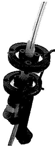
Figure 2.5: Implementation of an early ABS diaphragm design onto an iSprawl leg. Only two modules are shown connected to the leg. The outer frames are connected together via a section of rigid wire. This design was never tested during running, It was only implemented for feasibility purposes.
