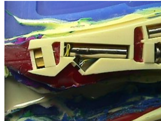
Detail of part just after inserting embedded components
