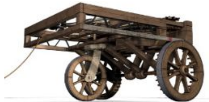
Da Vinci's programmable spring-powered cart
